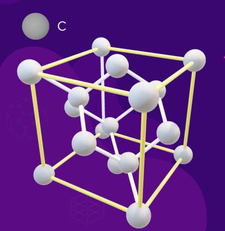
Diamond has ZnS type structure in which all  $S^{2-}$  location and all  $Zn^{2+}$  location are occupied by C atoms.
