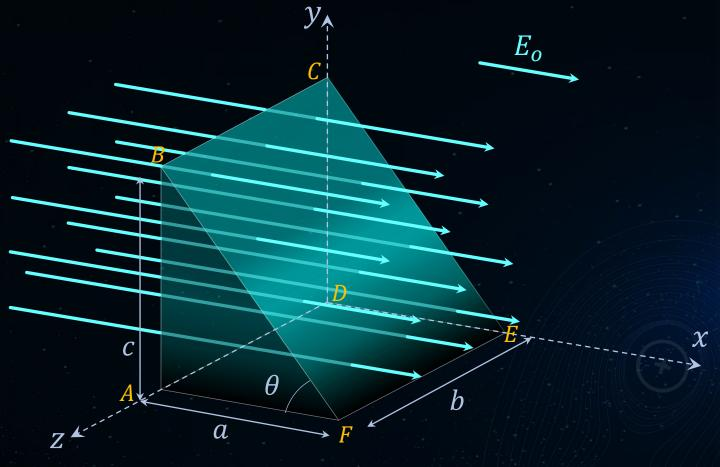
Since the surface ABF, CDF and ADEF are parallel to the electric field  $\vec{E}_o$  which means that the area vector of each of these surface will be perpendicular to the electric field. Therefore, the electric flux through these surfaces will be zero.
