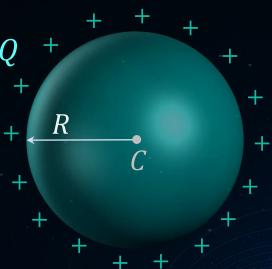
This potential energy is stored in the electric field generated by the sphere and in this case, the electric field extend from R to  $\infty$ .
